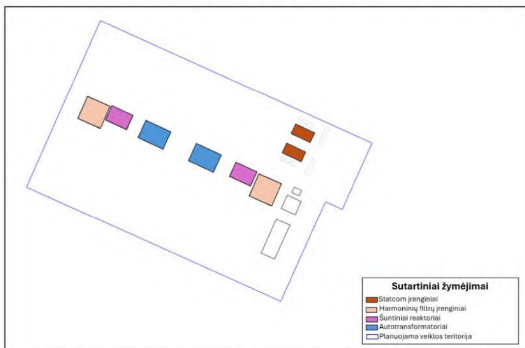
Fig. 3. Model of the layout of noise sources and project areas, created using the CadnaA software
